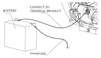
Use 12V and more than 36A.H battery, connect its positive lead to start relay terminal while connect its negative lead to engine mounting screw, base screw or other grounding point with the engine. (See Fig. 2)
